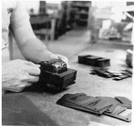
Figure 10.9b Stacking laminations inside a coil.
